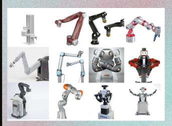
A collaborative robot or cobot is a robot that can safely and effectively interact with human workers while performing simple industrial tasks.
